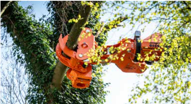
The actively controlled kinematics also enable lateral cuts.
