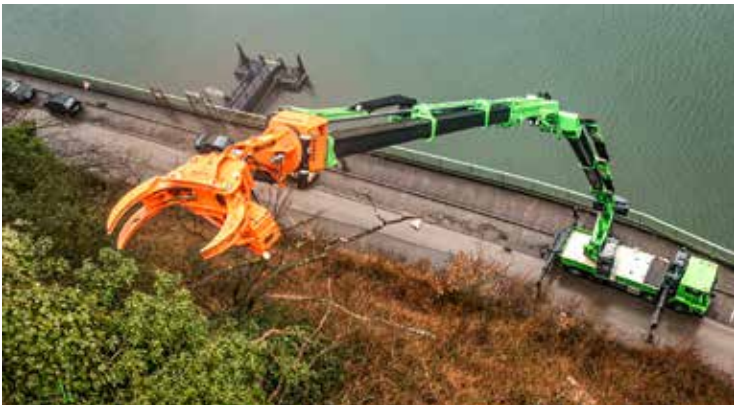
High reach for removals in the tree canopy and a large working radius.
