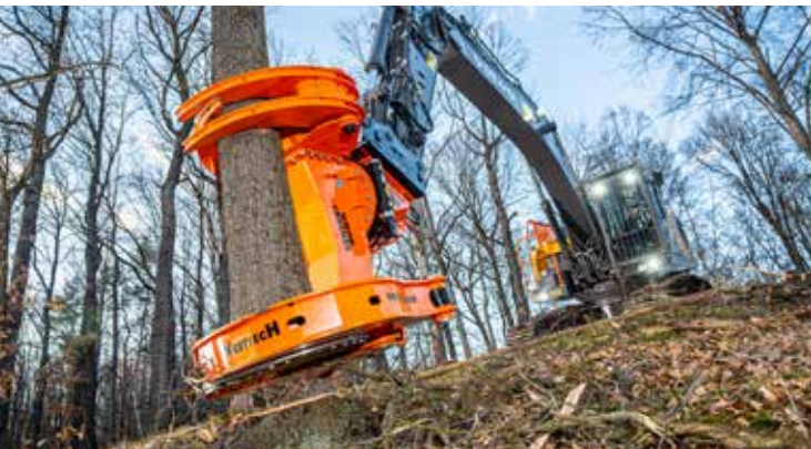
C650 with cutting diameter up to 70 cm.
