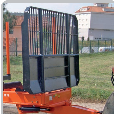
Frontal robusto con amplia visibilidad de carga. Robust front guard with high load visibility.
