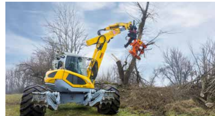
C300 with Menzimbuck walking excavator.
